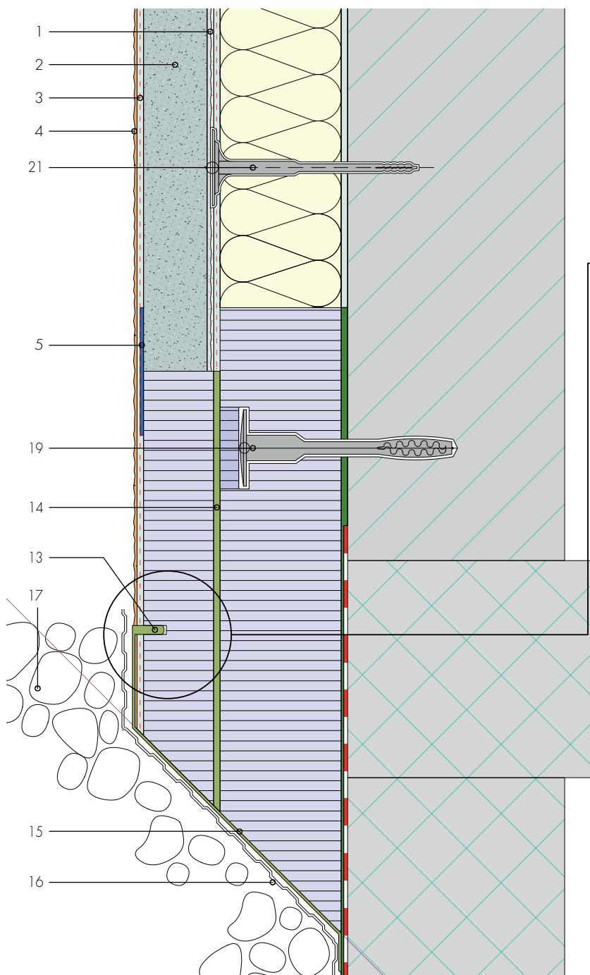
Detail of capillary slot 5 to 8 mm wide.
