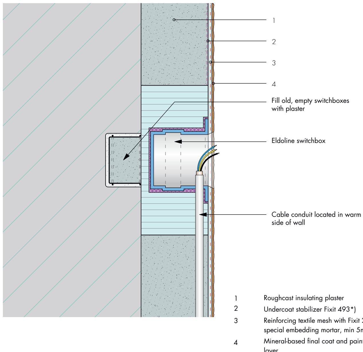
\*) only with Fixit 222 Aerogel Insulating Plaster
