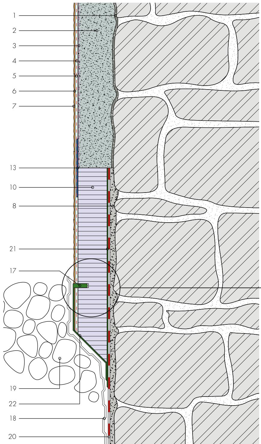
Detail of capillary break 5-8 mm, filled with Fixit 373 Multiflex base flagstone adhesive
